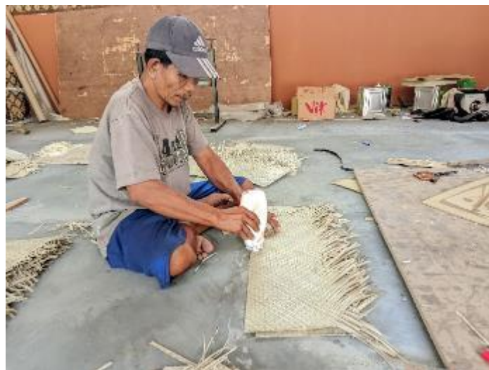
Fig.6. The process of gluing pandan weaving
